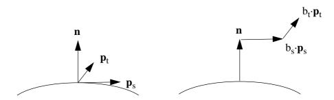
FIGURE 110. Bump mapping. The normal vector is modified by components in u and v direction
